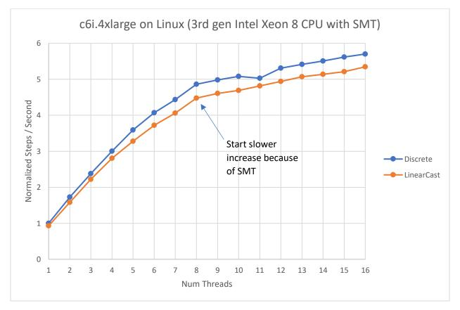
The graph above shows the amount of physics simulation steps per second normalized to 1 (1 core without CCD = 1). You can see that Jolt is 4.9x faster with 8 threads than it was with 1 thread. Using Simultaneous Multithreading (SMT) increases this to a 5.7x speedup with 16 threads. The system scales equally well with and without CCD although CCD (LinearCast) is obviously a bit slower.
