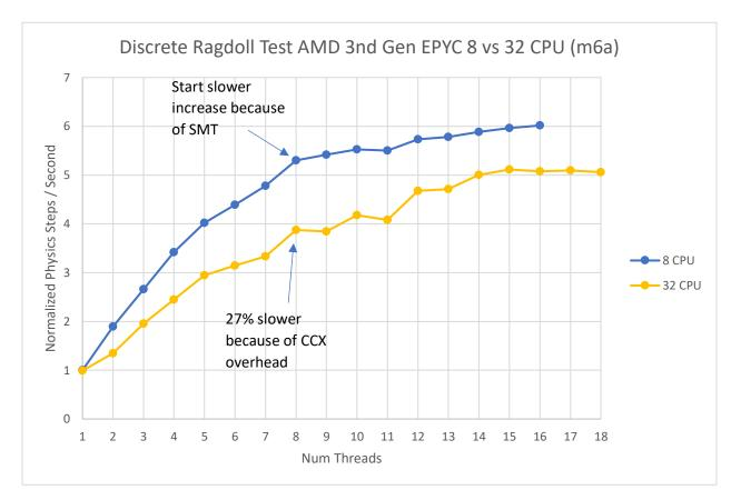
AMD processors consist of multiple Core Complexes (CCX). Memory operations (and especially atomic operations) cost a lot more when they cross CCX borders. Currently Jolt is not CCX aware. As you can see at 8 threads the simulation on 32 CPUs (4 CCX) is 27% slower than the same machine with 8 CPUs (1 CCX) just because jobs were scheduled at random across CCXs. To avoid this overhead, set the thread affinity of the job scheduler to use only a limited set of CCXs.
