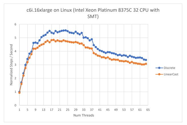
When going to extreme amounts of CPU cores we can see that Jolt does not scale infinitely.
