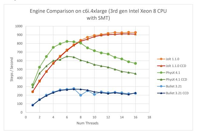
Repeating the test on an c6i.4xlarge with 8 CPUs shows that, for this scene, both PhysX and Bullet stop scaling at around 6-7 CPU cores:
